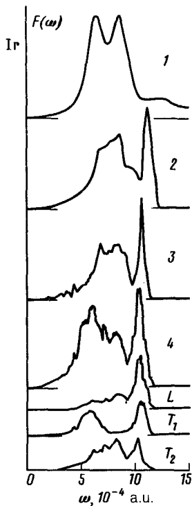
FIG. 1. Complete (1-4) and partial ( L, T_1, T_2 ) phonon state densities in Ir. 1—Present experiments; 2,3—calculations of Refs. 2 and 1, respectively; 4—present calculations of L, T_1 , and T_2 .
