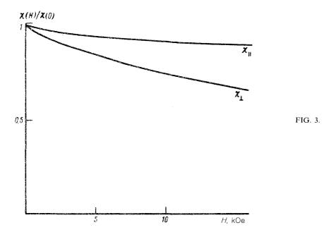
depends considerably on the orientation of the field (Fig. 3). In  $\sim$  10-kOe fields the ratio  $(\partial \chi_{\perp}/\partial H)(\partial \chi_{\parallel}/\partial H)^{-1}$  is 3.2 for sample 1. This ratio coincides within acceptable error margin with the ratio of the derivatives  $(\partial H_{c2\parallel}/\partial T)(\partial H_{c2\perp}/\partial T)^{-1}$  for the same sample, i.e., relation (1) holds. Relation (1) holds also for samples 2 and 3.
