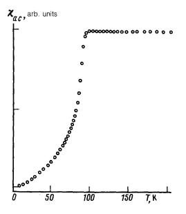
FIG. 1. Temperature dependence of the ac magnetic susceptibility,  $\chi_{ac}$  (T), of samples of the compound  $YBa_2Cu_3O_6Cl_x$ .
