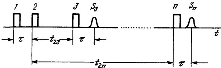
FIG. 1. Multipulse excitation of long-lived multiple optical echo signals. The numbers specify the order of the excitation pulse,  $n$ ;  $S_n$ , represents the echo signal.
