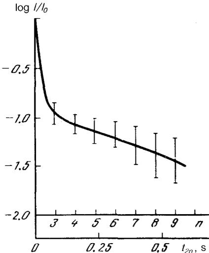
FIG. 3. Logarithm of the intensity of the long-lived multiple optical echo signal versus the number of the readout pulse. The pulse repetition frequency is 12.5 Hz.
