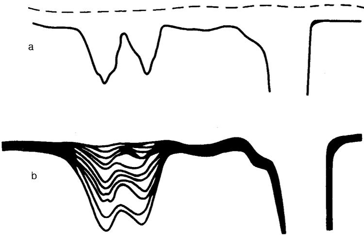
FIG. 2. Experimental oscilloscope traces. a: First and second writing pulses. The second pulse, which is the code pulse, is double humped. The time intervals between markers are 10 ns. b: Readout pulses and long-lived multiple optical echo signals. Successive pulses have been brought into coincidence along the time scale.
