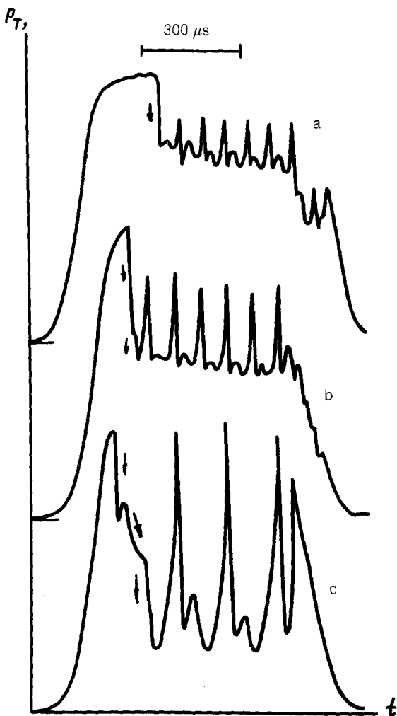
FIG. 2. Three states of strong absorption of a moving domain in the time evolution of the output signal, detected in the same geometry of the contracting optical channel with E \parallel C under the following experimental conditions: a— T = 240 K, P_0 = 780 mW; b— T = 248 K, P_0 = 640 mW; c— T = 248 K, P_0 = 960 mW.
