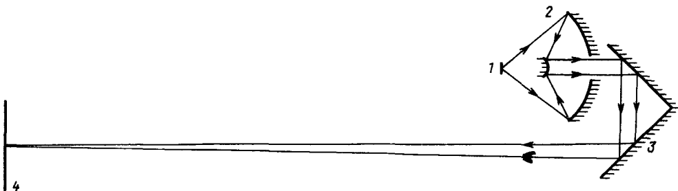
FIG. 1. Optical layout of the microscope. 1—Plane of object; 2—objective; 3—turning system; 4—plane of image.
