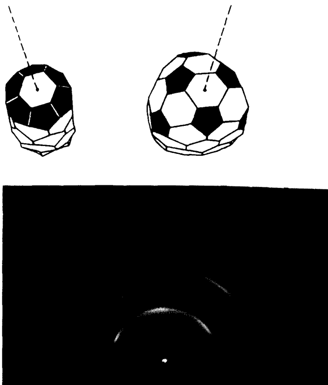
FIG. 3. Models of tube-like carbon clusters: the left one is C_{36+12n} with 0.48-nm cage diameter (the C axis of sixfold symmetry), the right one is C_{60+18n} with 0.72-nm cage diameter (the C axis of threefold symmetry). 3 At the bottom the electron diffraction patterns of the normal texture film (Fig. 2b) indicate mainly a sixfold symmetry of carbon located at its surface.
