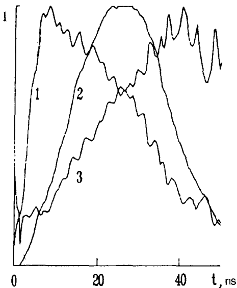
FIG. 3. Oscilloscope traces of the voltage U (1) and of the current I (2) in experiment 1047 at the PROTO-II device, along with a plot (3) of the total number of electrons in the gap, N_e(t) , in arbitrary units, constructed from these traces. The maximum voltage corresponds to 1.6 MV, and the maximum current to 2.4 MA.
