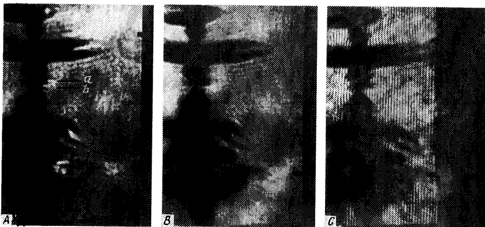
FIG. 1. Faraday (A), shadow (B), and interference (C) images of the plasma of an exploding 25\text{-}\mu\text{m} Al wire at the time at which a current of 100 kA is flowing through the wire and also at a time 13 ns before the beginning of x-ray emission.
