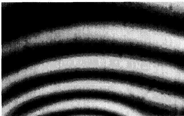
FIG. 3. Stripe state near a stripe source on a 420-layer film contour at T=49.5\text{ }^{\circ}\text{C} .
