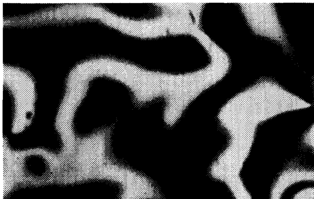
FIG. 5. Anisotropic texture of the smectic-C* phase in a mixture of 75% chiral C7 with its racemat, N=150 , T=53.85^\circ\text{C} .
