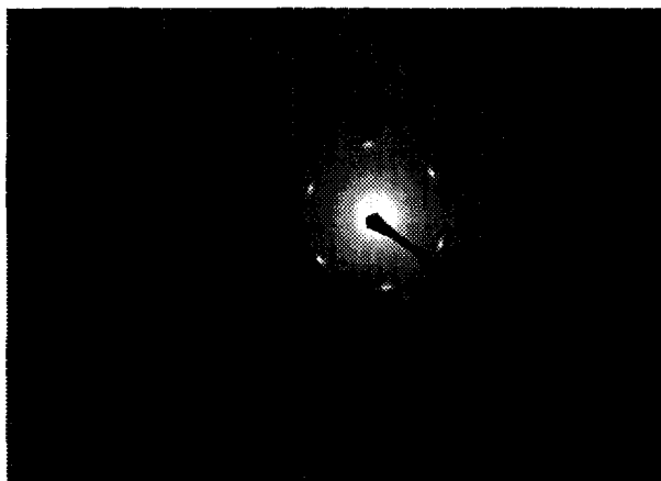
FIG. 1. Electron diffraction pattern from oriented close-packed carbon chains.
