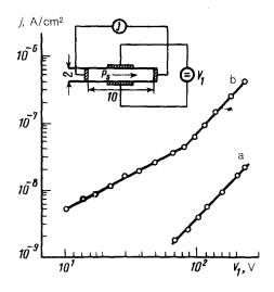
FIG. 1. Current-voltage characteristics of (a) the transverse current  $j_3$  and (b) the longitudinal current  $j_1$ . T = 300 K. The sample is a parallelepiped 10 mm long (the [001] direction), 2 mm high ([100]), and 5 mm wide ([010]). The longitudinal electrode has an area of  $4 \times 5$  mm<sup>2</sup>.
