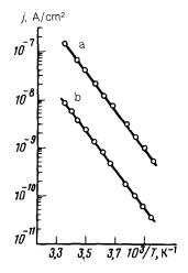
FIG. 2. Temperature dependence of (a) the transverse current  $j_3$ and (b) the longitudinal current  $j_1$ .  $E_1 = 1200$  V/cm.
