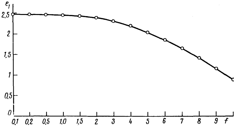
FIG. 2. The energy position of the first subband, e_1 , versus the normal component of the electric field, f(U_0=0) .
