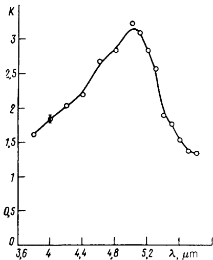
FIG. 2. Spectrum of the ratio ( K ) of emission coefficients of a copper grating and an aluminum mirror at the resonant angle \theta_{0P}^{\text{exp}}(l=1)=40.5^\circ .
