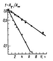
FIG. 1. Relaxation of longitudinal magnetization of liquid <sup>3</sup>He nuclei surrounding a TmES crystal at a temperature of 1.5 K:  $\triangle -\theta = \theta_x = 7.05^\circ$ ;  $T_1 = 2.4s$ ;  $\bigcirc$ ,  $\blacksquare = 7.5^\circ$ ; 6.5°;  $T_1 = 6.5s$ ;  $\theta$  is the angle between the *c* axis of the crystal and the external magnetic field.
