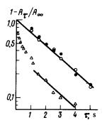
FIG. 2. Relaxation of the longitudinal magnetization of <sup>169</sup>Tm nuclei in a TmES crystal surrounded by a layer (~0.1 mm) of liquid <sup>3</sup>He at a temperature of 1.5 K;  $\triangle - \theta = \theta_X = 7.05^\circ$ ;  $T'_1 \sim 0.4$  s,  $T''_1 \sim 2.6$  s; O,  $\bullet - \theta = 7.5^\circ$ ; 6.5°;  $T_1 = 2.6$  s.
