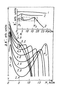
FIG. 2. a-Magnetic-field dependence of  $\chi'$  of the garnets MnGaG (1), CdCrG (2), and MnCrG (3); b-Magnetic-field dependence of  $\Delta\chi'$  (the part of curve 3 in Fig. 2a in the dashed box has been magnified by a factor of 15) for the garnet MnCrG.
