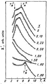
FIG. 1. Temperature dependence of the magnetic susceptibility of the garnets  $Mn_s Ga_x Cr_{2-x} Ge_3 O_{12}$ .
