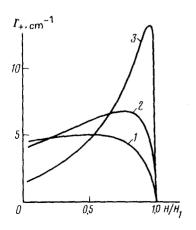
FIG. 1. Magnetic field dependence of the absorption coefficient of sound: curve 1, a = 0.5; curve 2, a = 1; curve 3, a = 3.
