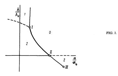
and 2. At the triple points I and II this line breaks up into two lines of the phase transitions. The lines of the first-order ferroelectric transitions 0-1 ( $\beta < 0$ ) and of the second-order transition 1=2 diverge at point I (if  $b \ge 1/4$ ). The lines of the improper, second-order ferroelectric transition 0=2 (b>0) and of the isostructural, first-order phase transition 2-2 diverge at point II which ends at point III (1/4  $\beta$  +3/5,  $-32\beta/25\sqrt{5}$ ).
