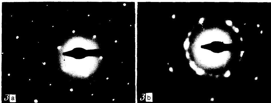
FIG. 3. Typical point (a) and ring (b) electron diffraction patterns of a C_{60} Langmuir-Blodgett film.
