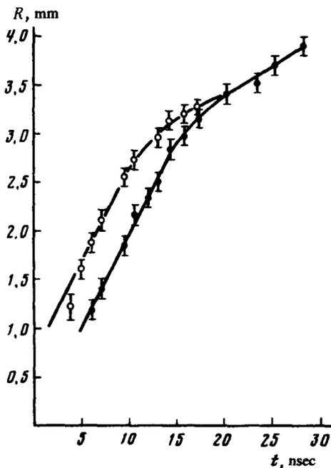
FIG. 2.  $R$ - $t$  diagram plots the propagation of the shock wave (curve 1) and of the ionization front (curve 2) in the initial stage.  $E_L = 60$  J,  $\rho_1 = 4 \times 10^{-6}$  g/cm<sup>3</sup>; the target is made of  $\phi$  140- $\mu$ m solid glass.
