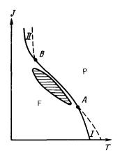
FIG. 1. Temperature-(illumination intensity) diagram of stationary states of the semiconductor. A self-excited oscillation occurs in the hatched region.
