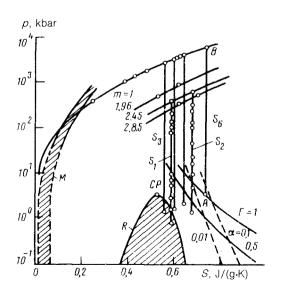
FIG. 2. Entropy diagram of bismuth. M—Melting region (at low pressures, the melting of the metastable high-pressure phase BiVI is shown, because of the complex picture of structural transitions in bismuth); R—line of the liquid-vapor equilibrium with the critical point (CP);  $\alpha$ —degree of ionization;  $\Gamma$ —the Coulomb collisionality parameter. The notation is otherwise the same as in Fig. 1.
