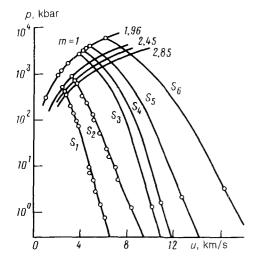
FIG. 1. Dynamic experiments on the highenergy states of a dense bismuth plasma. p, u-The pressure and mass velocity in bismuth samples during shock-wave loading and in the isentropic decompression waves; m-shock adiabats of samples with various initial porosities; S-decompression isentropes. Points—experimental; solid lines-calculated.
