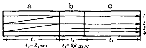
FIG. 1. Passage of acoustic pulses through a sample (b); a and c—the transmitting and receiving piezoconverters.
