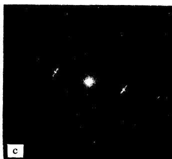
FIG. 2. (a) k_r —Projection of the vector of the reflected wave; u_{\pm} —two opposite directions of motion of a spot. The dashed line shows the kinematics of formation of a degenerate grating q_3 . (b) Reflections from the grating q_2 . (c) Reflections from the grating q_1 .
