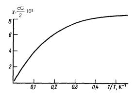
FIG. 1. Temperature dependence of the magnetic susceptibility of BIPO.
