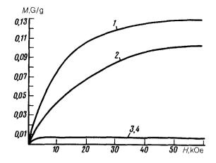
FIG. 2. Magnetization of polyBIPO versus the magnetic field at various temperatures: 1-1.7; 2-4.2; 3-25: 4-90 K.
