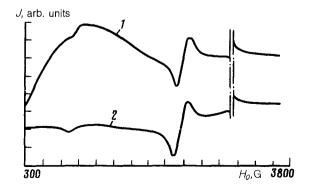
FIG. 3. ESR spectra of polyBIPO in two arrangements. 1-Parallel to the field; 2-perpendicular to the field.
