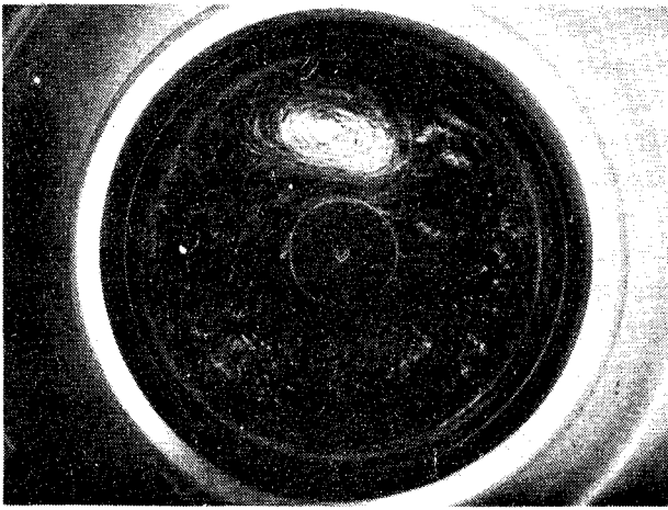
FIG. 1. Representative visualization of a Rossby autosoliton (top view). The center of the layer of shallow water is rotating more rapidly than the periphery. The white lines are tracks of tracer particles floating on the surface of the liquid, seen against the black bottom of the paraboloid ( \Omega_0 = 12.6 \text{ s}^{-1} ; the camera exposure time is 1/3 \text{ s} ; the distance from the center of the vortex to the rotation axis is about 6 cm).
