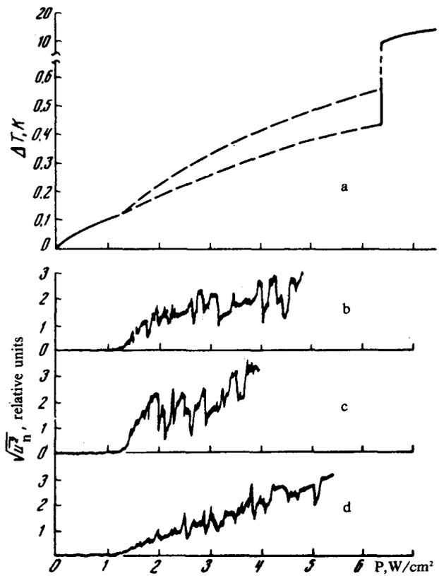
FIG. 2. Dependence on the intensity of the exciting light: a of the superheating of the germanium crystal relative to the helium bath,  $T_B = 2.07$  K; b of the noise of the scattered light; c of the noise of the electrical conductivity,  $E = 1$  V/cm; d of the noise due to absorption of the microwave radiation with  $\lambda = 2$  mm. The immersion depth of the sample in the helium bath is 15 cm.
