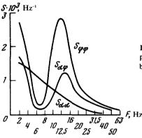
FIG. 2. Spectral density of intensities of amplitude  $S_{\alpha\alpha}$ , phase  $S_{\phi\phi}$  and reciprocal  $S_{\alpha\phi}$  fluctuations calculated on the basis of results in Fig. 1.
