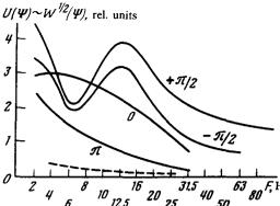
FIG. 1. Fluctuation spectra for four phase values of interfering waves  $\psi=\pm\pi/2,0,\pi$ . The dotted line indicates the shot noise level, F—average channel frequency.
