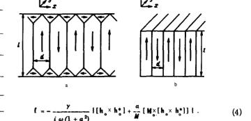
If the field h is linearly polarized, then f=0. If h is circularly polarized in the xy plane, then f has in the case of small damping only a z component,  $f_z = (1/2)\gamma h_0^2/\omega$ . In such a field, an additional pressure is exerted on the domain walls by the difference between averaged energy densities in the domains with opposite methodizations.
