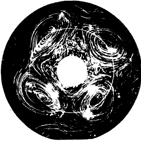
FIG. 2. Excitation of the fourth mode of the Kelvin-Helmholtz instability. The line of discontinuity in the flow velocity passes through the center of the vortices.
