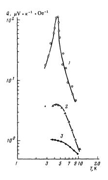
FIG. 1. Temperature dependence of the Nernst coefficient for Bi,  $H \| C_3$ , 1,  $\gamma_1 = 625$ ; 2,  $\gamma_2 = 344$ ; 3,  $\gamma_3 = 147$ .
