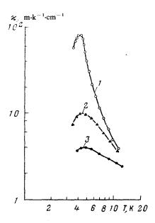
FIG. 2. Temperature dependence of the thermal conductivity of the same samples. The curves are numbered just as in Fig. 1.
