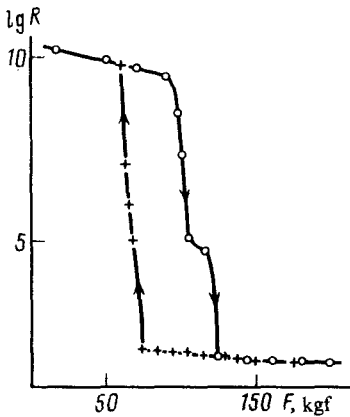
FIG. 2. Load dependence of electrical resistance for magnesium oxide. The indenter tip angle is 168^\circ . The initial layer thickness is \sim 0.01 mm and the average layer thickness under indenter after several compression cycles is \sim 1 \mu\text{m} . The average pressure at the point of abrupt decrease in resistance is \sim 30 kbar.
