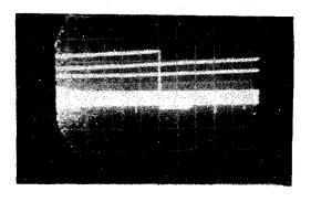
FIG. 2. Resistance of the pressure sensor as a function of time. The scale is 2 msec/div. The lines of slow increase and rapid release of the pressure are visible.
