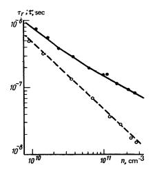
FIG. 1. Dependences of the lifetime (o) and of the relaxation time ( $\bullet$ ) of the submillimeter photoconductivity for the binding of carriers into excitons on the free-carrier density n (T=4.2 K).
