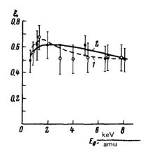
FIG. 2. Relative fraction of 2p-1s transitions  $\xi = \sigma(2p-1s)/\sigma(nl-1s)$ , plotted as a function of the collision energy for  $C^{6+}$ -H<sub>2</sub> (curve 1) and  $O^{8+}$ -H<sub>2</sub> (curve 2).
