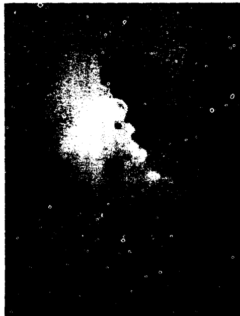
FIG. 3. Photocondensation of iodine in light beam. Magnification \sim 70\times .
