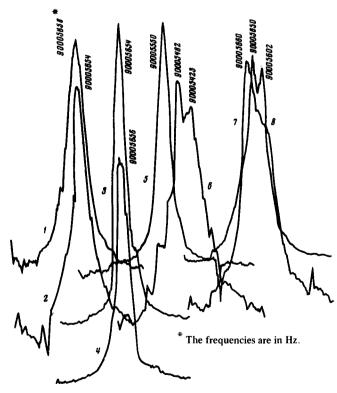
NMR spectra of protons in thin films of water or solution between various surfaces: each pair of curves pertains to two mutually perpendicular azimuthal orientations in a magnetic field parallel to the film: 1,2-water (thickness 20  $\mu$ ) between teflon surfaces; 3, 4-the same between glass surfaces; 5,6-KNO<sub>3</sub> solution (thickness 15-20  $\mu$ ) between (010) faces of KNO3; 7,8-solution between (100) faces of NaNO2.
