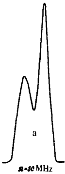
FIG. 2. Waveform of generation line at a pump-wave frequency detuning \Omega \approx 50 MHz.
