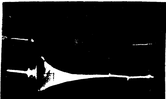
FIG. 1. Oscilloscope traces of the radial (upper trace) and vertical (lower trace) oscillations. The sweep rate is 5 ms/div; I = 100 mA; \epsilon = 70 MeV, p_0 = 5 \times 10^{-8} Torr.
