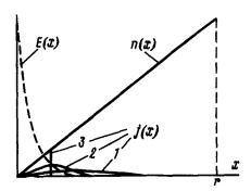
FIG. 1. Dynamics of the current density profile j(x) during the electron acceleration. Curves 1, 2, and 3 correspond to successive stages in the acceleration.
