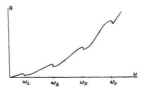
Formula (6) shows that at the resonance points ( $\omega=\omega_n$ ) the derivative dQ/d $\omega$  becomes infinite on the low-frequency side,  $\omega<\omega_n$ . The weakness of the singularity is due to the fact that it is determined only by the electrons of the limiting point, at which  $v_z=v_F$  (see below).
