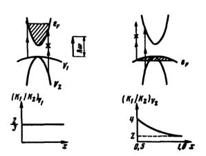
Scheme of possible two-photon transitions in indium antimonide: a)  $n_0 = 6.2 \times 10^{17}$  cm<sup>-3</sup>,  $\lambda = 9.5$   $\mu$ ; b)  $p_0 = 1.1 \times 10^{18}$  cm<sup>-3</sup>,  $\lambda = 10.6$   $\mu$ ;  $T = 77^{\circ}$ K.
