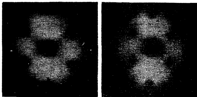
Fig. 1. Field-emission electron micrograms of needles: a) initial, b) elongated by the field ("sharpened") and annealed.
