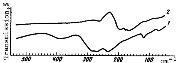
Fig. 1. IR transmission spectra of germanium monochalcogenides: 1 - GeS, 2 - GeSe.
