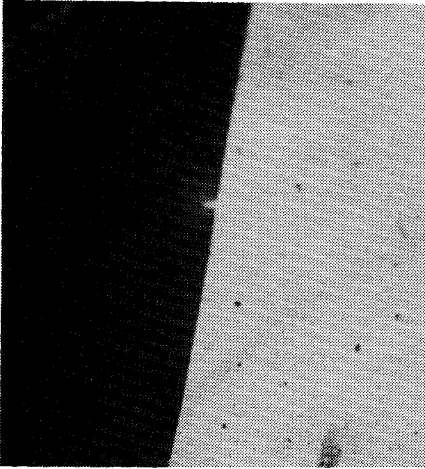
FIG. 1. Domain structure in YFeO 3 , plate perpendicular to the optical axis in a magnetic field with a gradient 500 Oe/cm directed along the a axis. Plate thickness 80 μm, magnification 30×.
