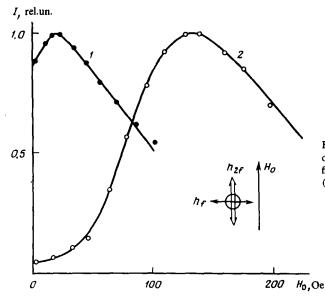
FIG. 2. Dependence of the intensity of the echo on the external magnetic field for unenriched (1) and enriched (2) samples.
