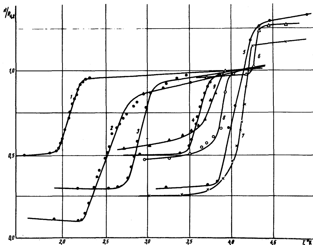
Fig. 1. Change of electric resistivity of tellurium samples going over into the superconducting state in the pressure range 40 - 100 kbar. Te II: 1 - 43, 2 - 48, 3 - 53, 4 - 61, 5 - 66 kbar. Te IV: 6 - 84, 7 - 88, 8 - 96, 9 - 100 kbar.
