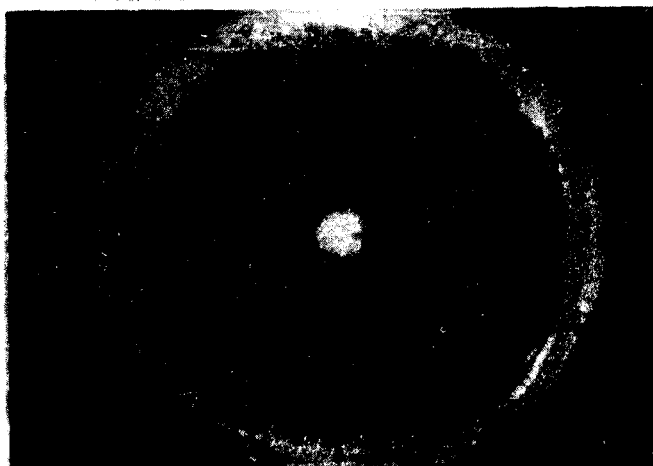
Fig. 1. Picture observed when a neodymium laser beam is incident on a metanitroaniline crystal perpendicular to the cleavage plane.
