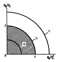
Growth increment of the spin wave as a function of the external fields Ho and eo. Curves a, b, and c correspond to increments  $\kappa = -\gamma/2$ , 0, and  $\gamma/2$ . The stability region is cross hatched.
