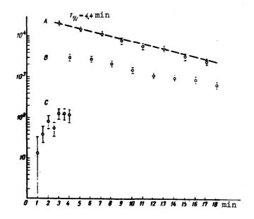
Change of intensity of the 148-keV line of 92 Tc with time: A - in the technetium fraction, B and C - in the ruthenium fraction. The time marked on the abscissa axis is reckoned from the instant of termination of the chemical separation of the corresponding fractions.
