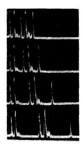
A series of two exciting microwave pulses of duration on the order of 3  $\times$   $10^{-8}$  sec and with an interval  $\tau$  between pulses was fed to the input of a three-arm ferrite circulator and further into a reflecting cavity resonator with a loaded Q on the order of 500.
